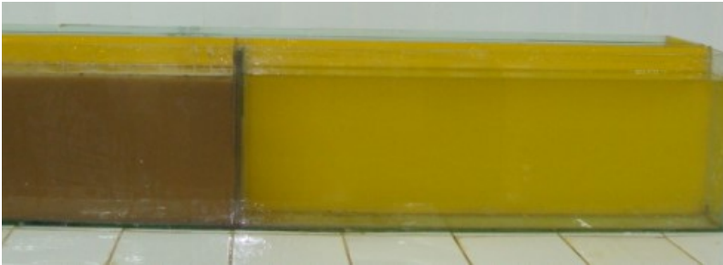
a) Contact between charged water and salt water
