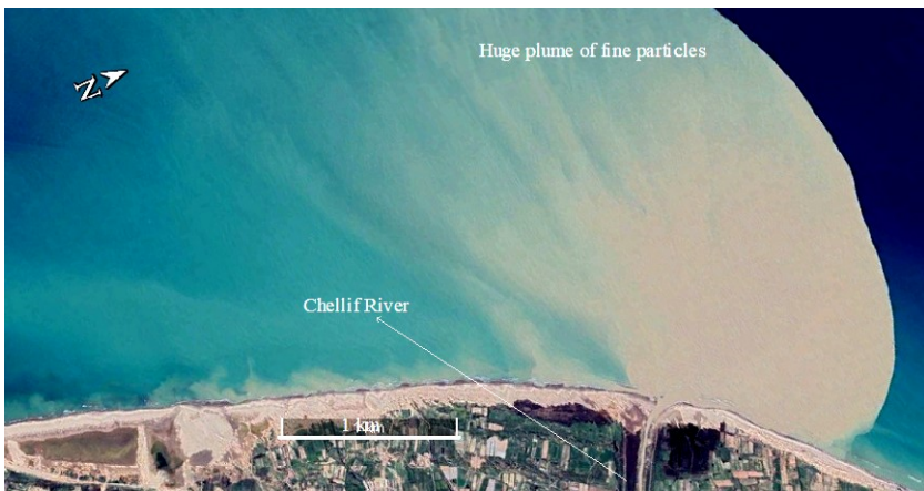
Figure 9: Chellif River March 2014. Enormous propagation of the fine particle plume out to sea (Google Earth)
