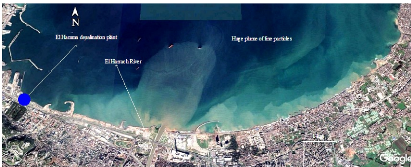
Figure 12: El Harrach River - Flood of May 2018. The Bay of Algiers is occupied by an immense plume of fine particles that even threatens the seawater collection tower of the El Hamma desalination station (Google Earth).
