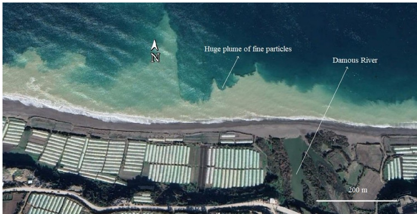
Figure 15: Releases from the Kef Eddir dam in January 2021 - Formation of an immense plume of fine particles (Google Earth)
