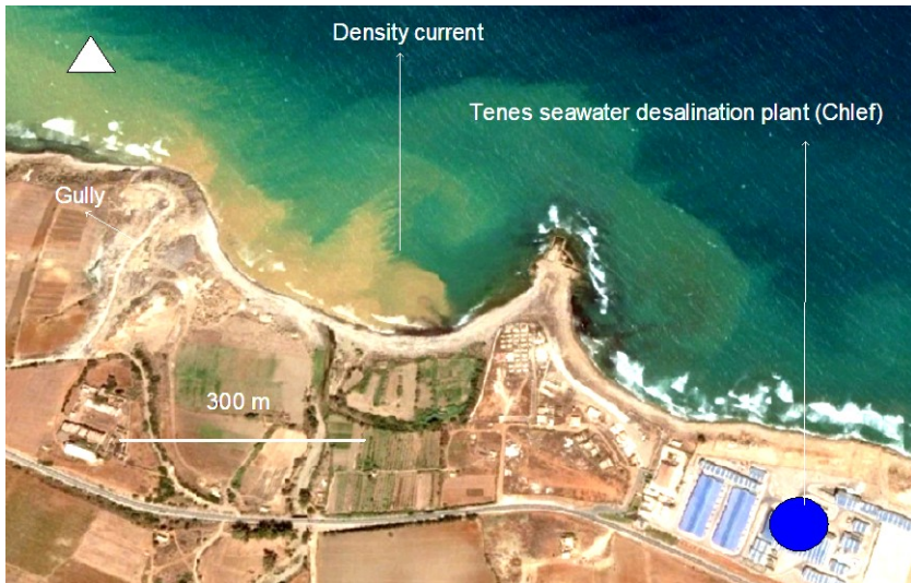
Figure 13: Flood of September 2016. Ténès seawater desalination station. A gully can trigger an immense plume of fine particles, and consequently, the raw water becomes of poor quality (Google Earth)
