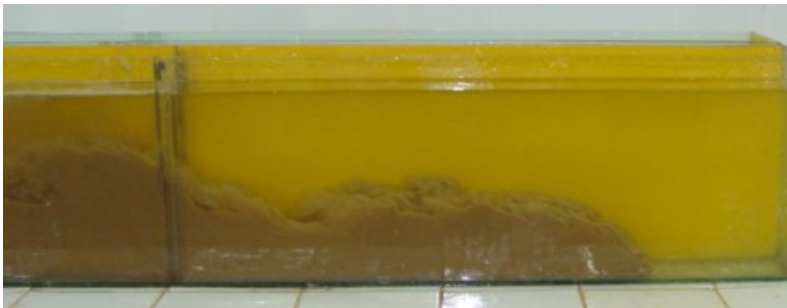
c) Propagation of a density current
