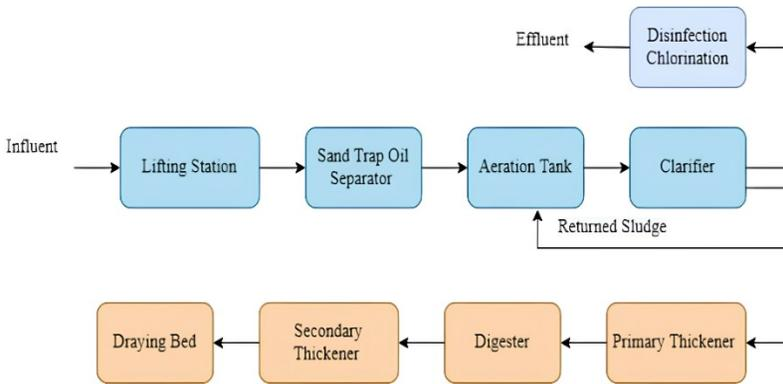
**Figure 2: Process scheme of the Ain Beida WWTP**
