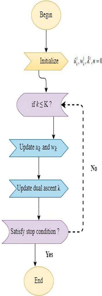
**Figure 11: Flowchart of the VMD method**
