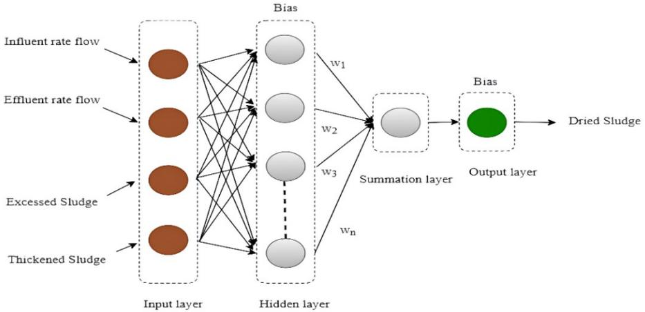
**Figure 7:** Schematic representation of the GRNN model for predictive modeling of DS
