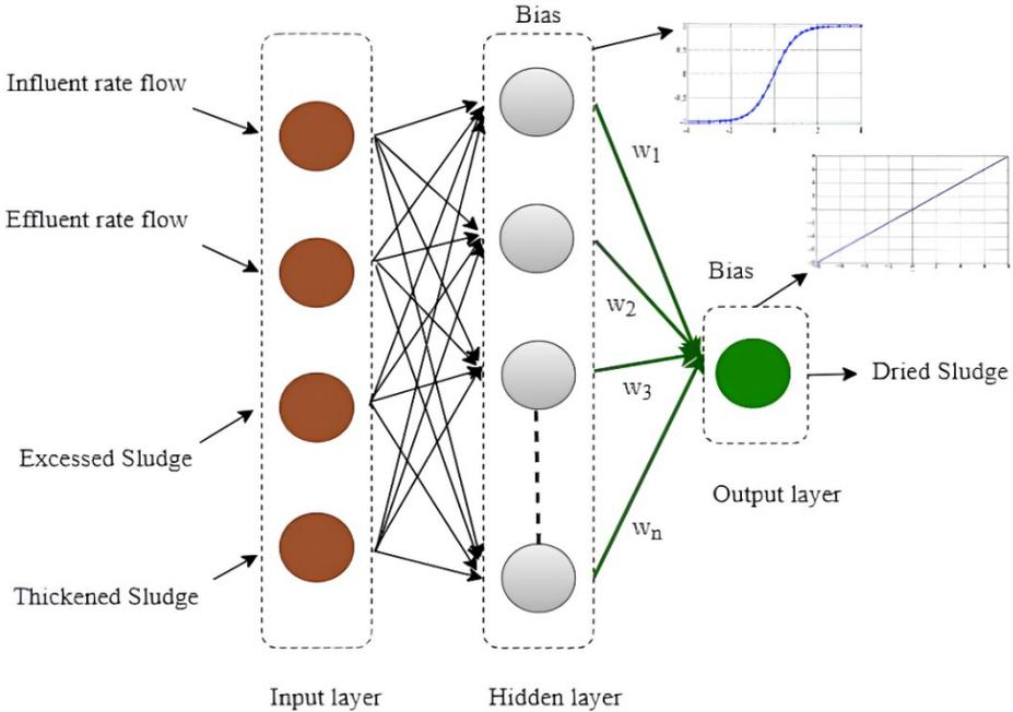
**Figure 5: Schematic representation of the MLPNN model for predictive modeling of DS**
