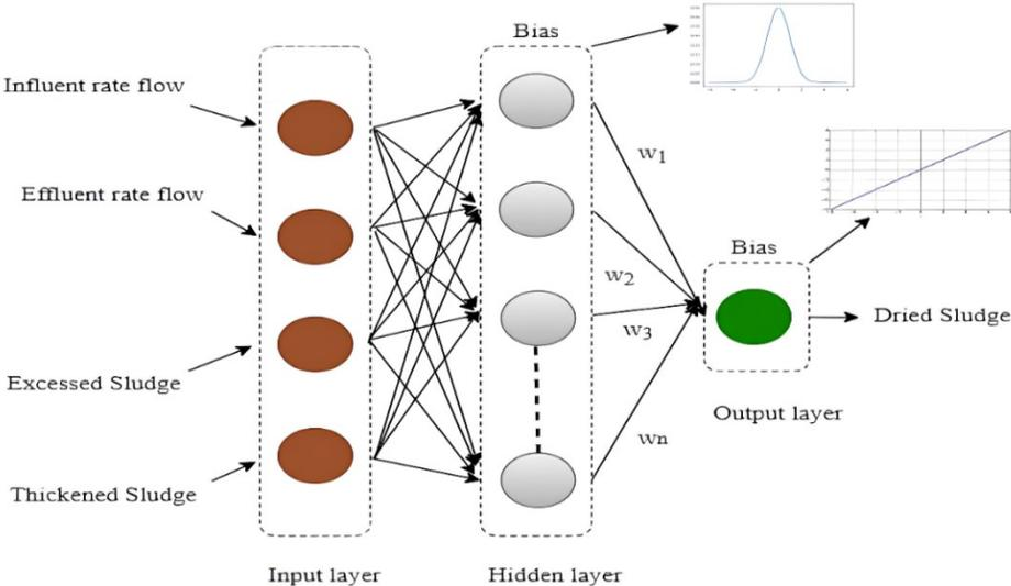
**Figure 6: Schematic representation of the RBFNN model for predictive modeling of DS**
