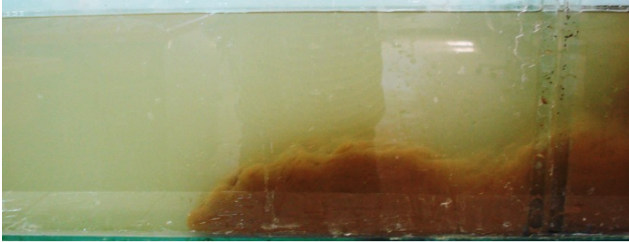
Figure 26: Propagation of density current in a rectangular channel (Photo Remini, 2015)
