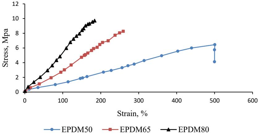
Figure 1: Uniaxial Tension Test Results of EPDM 50, 65 and 80
