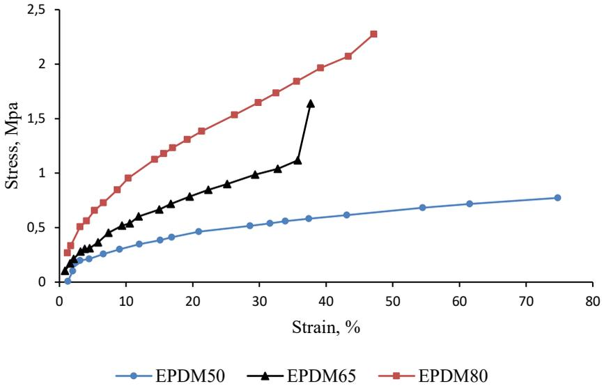
Figure 3: Planar Shear Test Results of EPDM 50, 65 and 80
