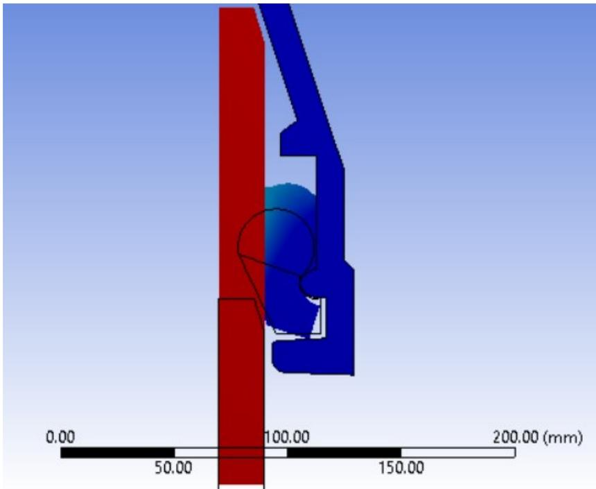
**Figure 7: Converged Solution of a Gasket Joint with a Deformed Gasket**
