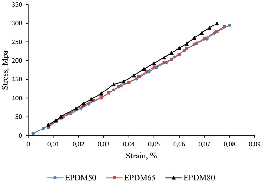
Figure 4: Volumetric Compression Test Results of EPDM 50, 65 and 80
