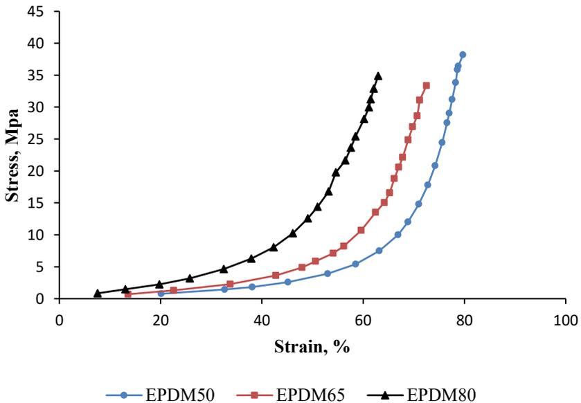
Figure 2: Uniaxial Compression Test Results of EPDM 50, 65 and 80
