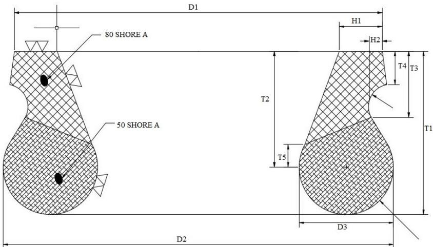
**Figure 5: Drawing of a TJ-type Gasket**
