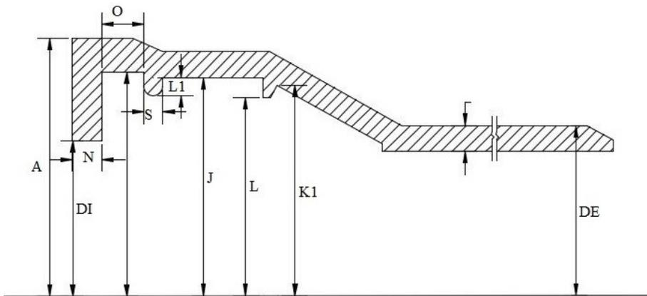
**Figure 6: Drawing of the Socket Component of the Joint**
