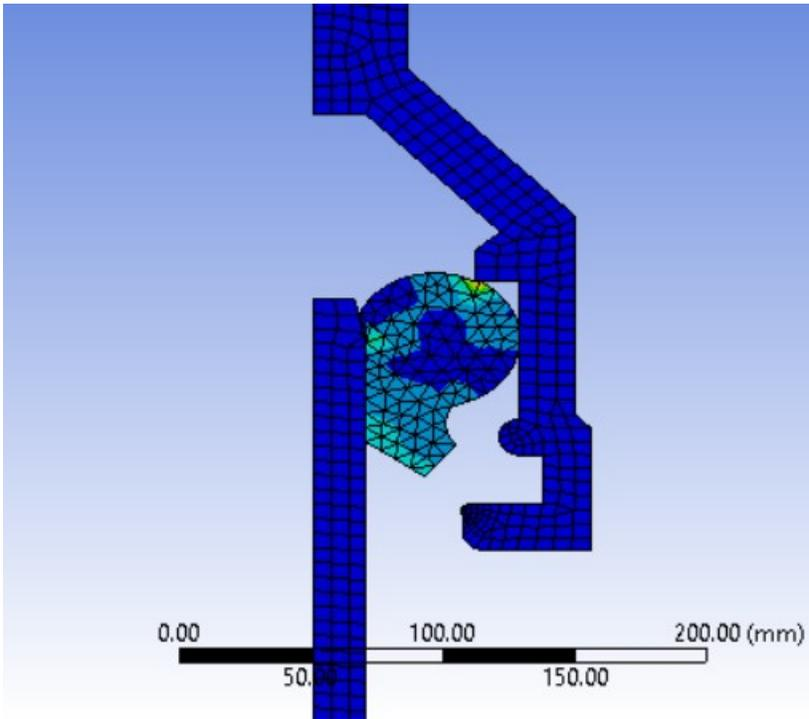
**Figure 8: Unconverged Solution of Joint with Gasket not Fully Deformed**
