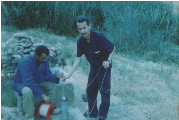
Photograph 5: Water Removal from Piezometers on the Left Bank of the QuizertDam (Benfetta, 2018)
