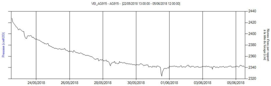
Figure 6: Water level variation compared to the borehole SIF4's head
