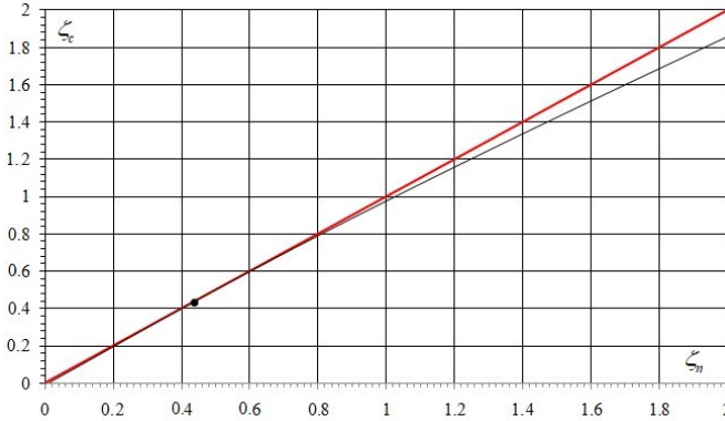
Figure 4: Variation curve of \zeta_c depending on \zeta_n in a smooth parabolic channel for a slope S_0 = 0.0023624406 , (•) single critical flow state, \zeta_c = \zeta_n \approx 0.451 .
