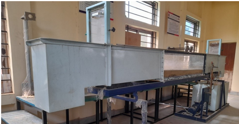
Figure 3: Experimental set-up of the Tilting flume used in the study
