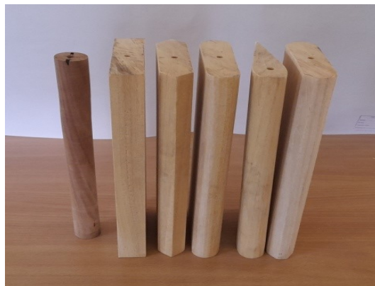
Figure 4: Various bridge pier types utilized in the experimental study. (Circular, rectangular, sharp-nosed, oblong, Joukowski, and chamfered shapes)
