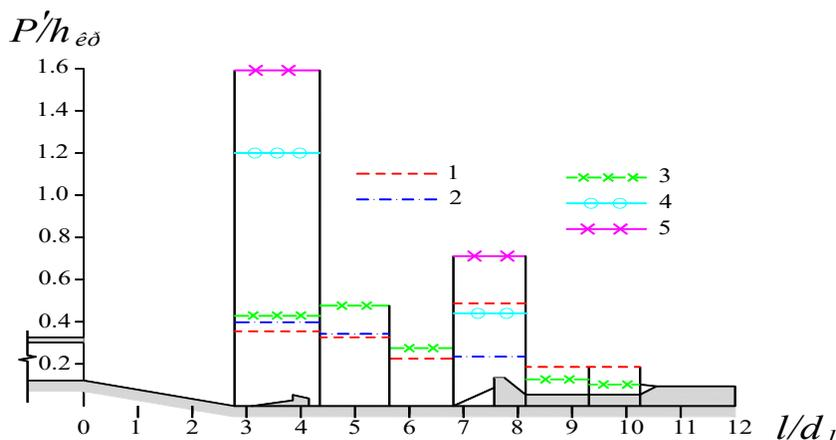
**Figure 7: Comparison of specific averaged pulsation loads  $P'_o$  on the socket bottom fastening plates: 1 -  $P'_o$  according to data from (Lappo, 1988) for mode 1; 2 and 3 - experimental data during the operation of all three galleries  $P'_o$  and  $P'_{om}$ ; 4 and 5  $P'_o$  and  $P'_{om}$  when the structure operates only on the middle span**
