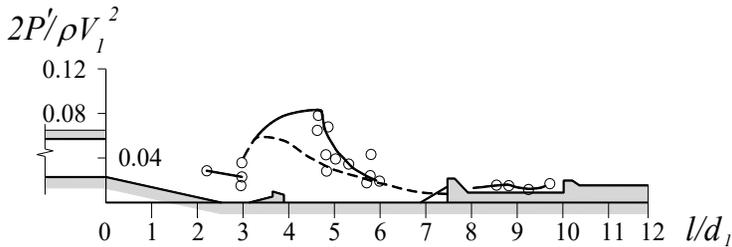
**Figure 5: Change in the relative standard of pressure pulsation  $2P'/\rho v_1^2 = P'/\gamma v^2 / 2g$  (where  $\rho = \gamma/g$  is the density of water) at the points of attachment of the bottom of the bell section behind the spillway when all three galleries are operating (mode 1)**
