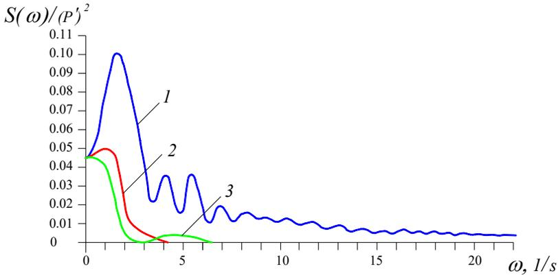
**Figure 8: Functions of the spectral density of pressure pulsations and loads on the slabs of the water breaker behind the first row of dampers when the spillway operates in three galleries (mode 1): 1 –  $S(\omega)$ ; 2 –  $S_M(\omega)$ ; 3 –  $S_p(\omega)$**
