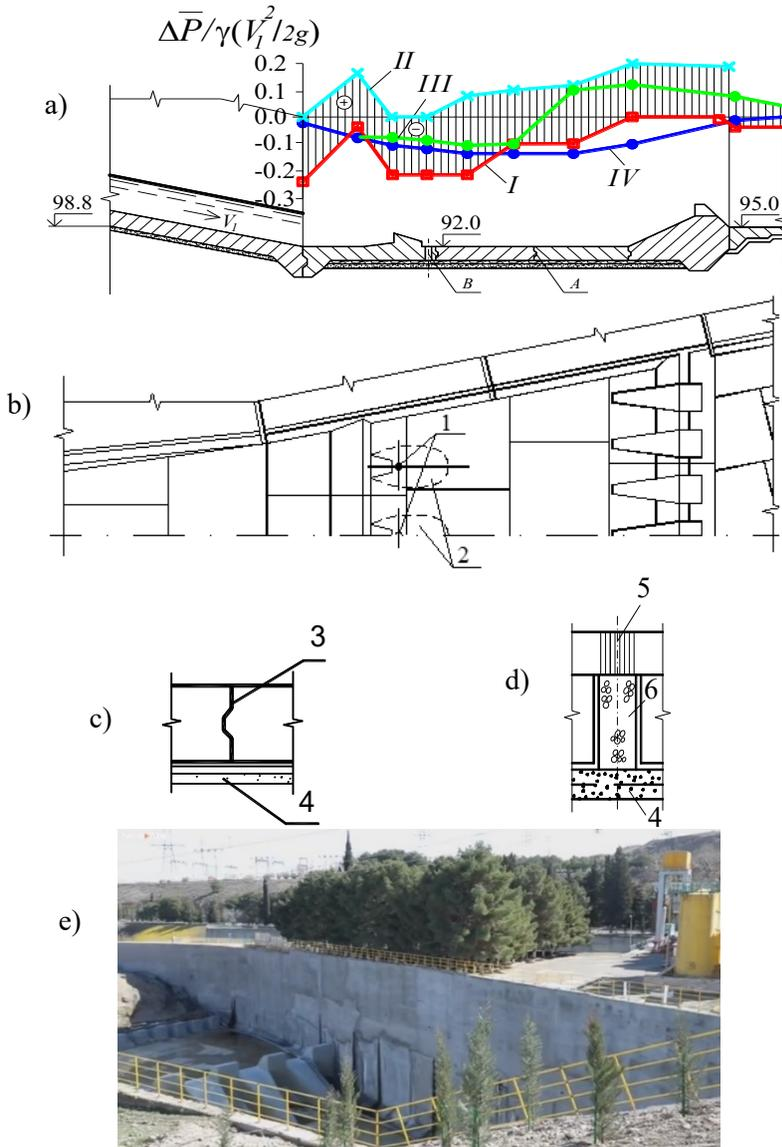
**Figure 4: Scheme of quasi-static loading and the proposed structural elements of the fastening slabs of the water outlet section of the Shamkir hydroelectric complex:**
