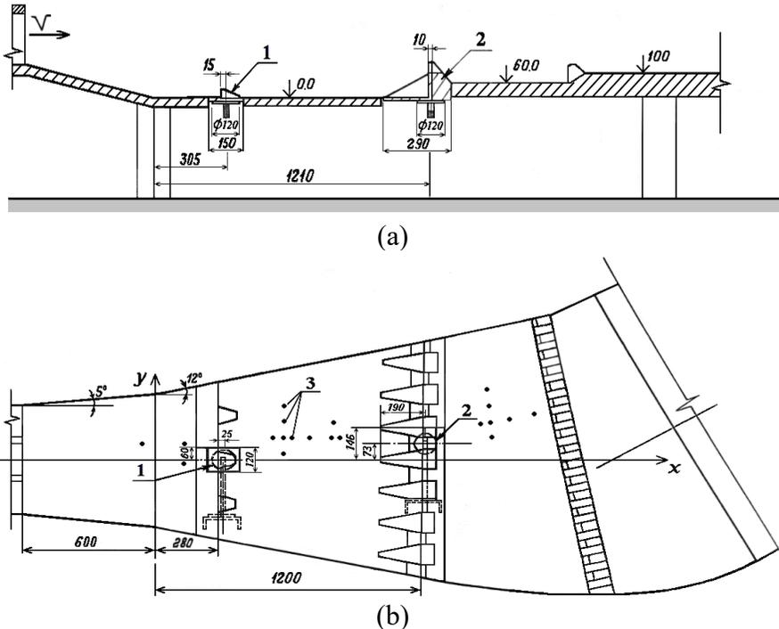
**Figure 3: Installation diagram of sensor dampers (1) and point sensors (2) on the spillway model of the Shamkir hydroelectric complex: a) longitudinal section along the axis of the outlet head; b) plan of the exit section**
