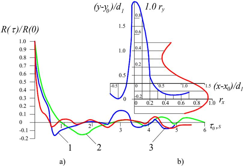
**Figure 6: a) Spatial correlation; b) types of autocorrelation functions of pressure pulsations at different points along the axis of the bottom of the water well. 1 – in front of the first row absorber; 2 – in the middle of the water hole, between the first and second rows of dampers; 3 – behind the second row of dampers**
