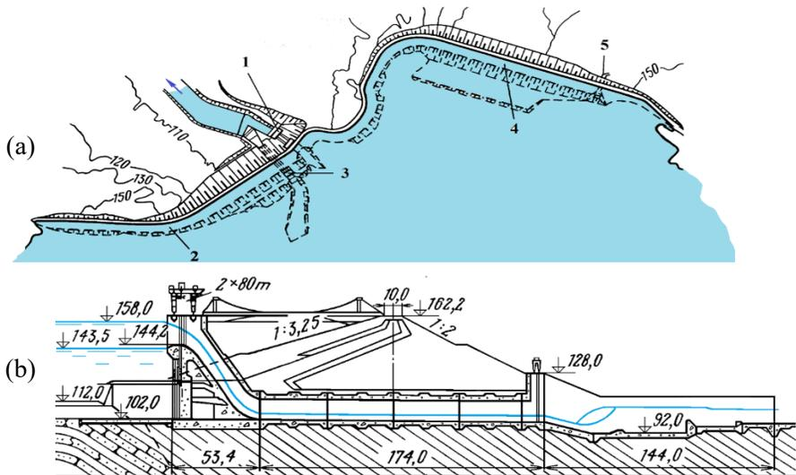
**Figure 1: Plan of the Shamkir hydroelectric complex. (a) and longitudinal section along the operational spillway (b)**
