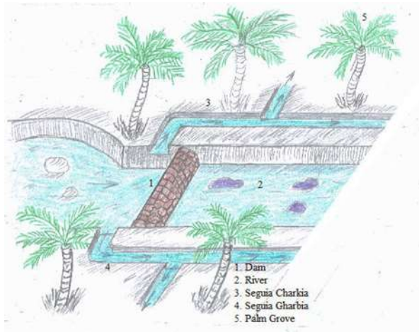
Figure 9: Synoptic diagram of the spring dam system (Diagram Remini, 2025)
