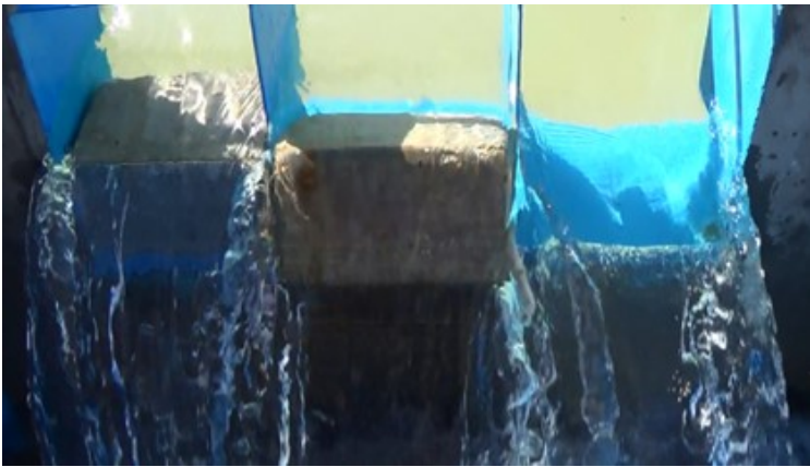
Figure 8: Downstream view of the flow over the fuse plugs at the moment the central block overturns
