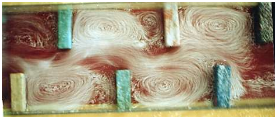
Figure 34: The staggered shape of the obstacles in a wadi is the best arrangement for accelerating the recharge of the alluvial aquifer (Photo. Remini, 2004).
