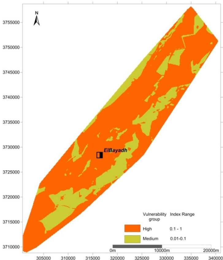
**Figure 9: Vulnerability classes obtained with the proposed methodology mapped for the ElBayadh aquifer**
