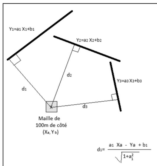
Figure 3: Mathematical function used to determine fracturing density
