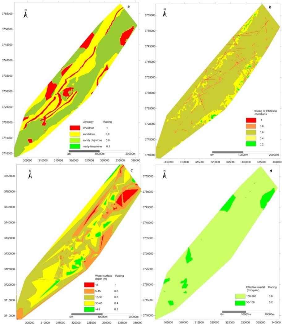
**Figure 7: Vulnerability factors maps: a-lithology, b-infiltrations conditions, c- depth to groundwater surface and d-effective rainfall**
