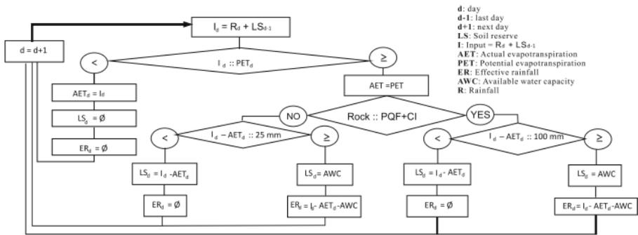
Figure 8: Flowchart enabling calculation of AET and ER (Modified) (Yousfi et al. 2013)
