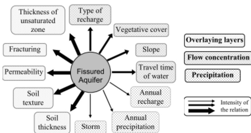
**Figure 1 : Influence of main variables and factors on the resource vulnerability of fissured aquifers (Vías et al. 2006).**
