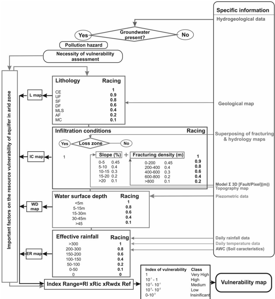
Figure 5: Model used to determine the groundwater vulnerability in arid zone
