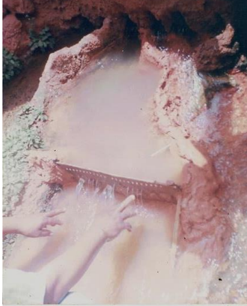
Figure 41: Operation of measuring the flow of the foggara of El Meghier by the louh (Photo. Remini 2007)
