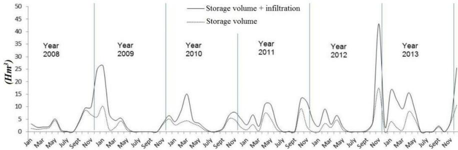
**Figure 6 : Graphical representation of water balance and infiltration of Meffrouch dam**
