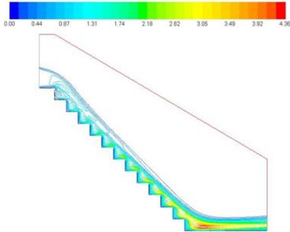
**Figure 9: Contour map of turbulent viscosity for  $q=0.22 \text{ m}^2\text{s}^{-1}$ .**
