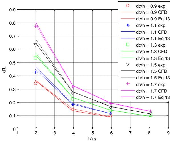
**Figure 6: Comparison between equation (13) and normalised water depth obtained by experimental (exp) and by Ansys Fluent (CFD)**
