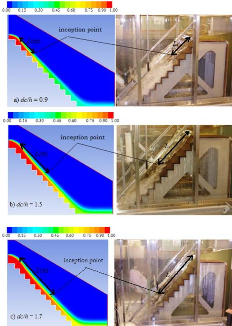
**Figure 3: Free surface obtained by Ansys Fluent**
