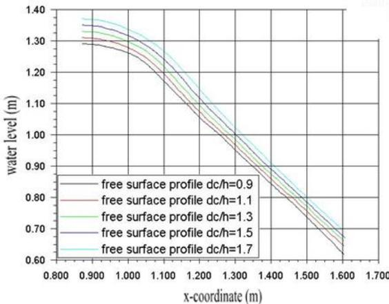
**Figure 4: Free surface obtained by Ansys Fluent**
