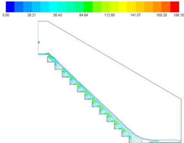
**Figure 10 : Vorticity along the stepped spillway for  $q=0.22\text{m}^2 \text{ s}^{-1}$**
