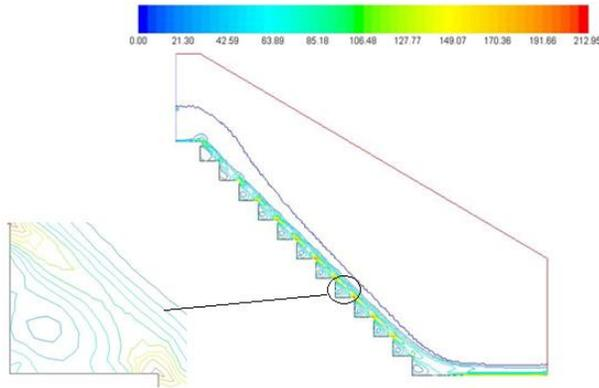
**Figure 11: Shear strain rate along the stepped spillway for  $q=0.22\text{m}^2 \text{s}^{-1}$**
