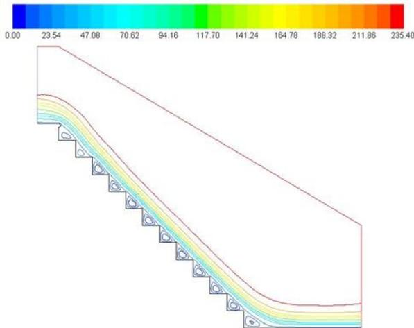
**Figure 8: Stream function along stepped spillways for  $q=0.22\text{m}^2\text{ s}^{-1}$**
