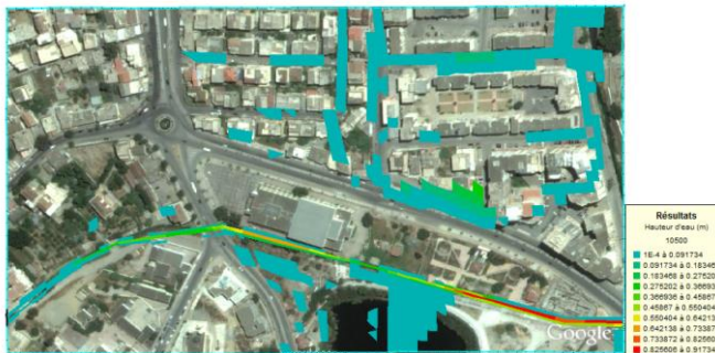
Figure 9: Water heights of water in t = 10500 sec for a flood of 10 years return period
