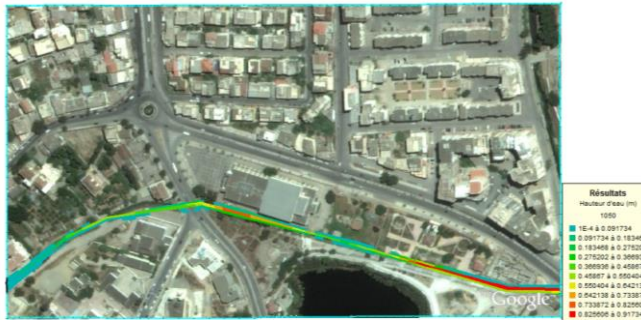
Figure 3: Water heights in t = 1050 sec for a flood of 10 years return period
