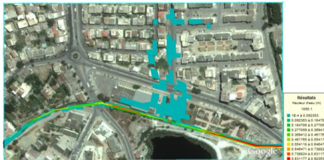
Figure 4: Water heights in t = 1050 sec for a flood of 20 years return period
