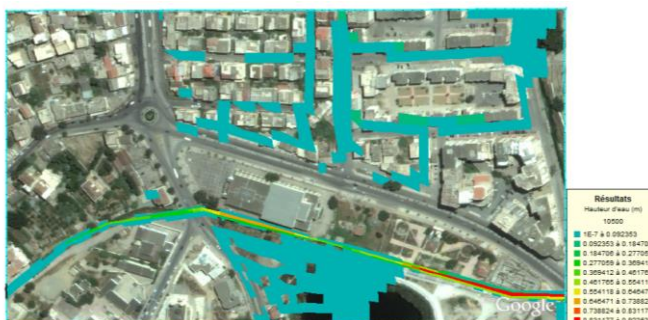
Figure 10: Water heights in t = 10500 sec for a flood of 20 years return period
