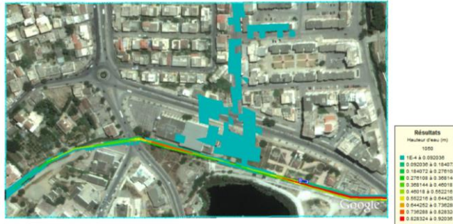
Figure 5: Water heights in t = 1050 sec for a flood of 25 years return period
