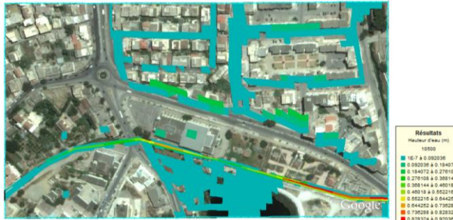
Figure 11: Water heights in t = 10500 sec for a flood of 25 years return period
