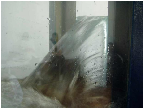
Photo 3: Side view of the contracted flow crossing the notch of the device
