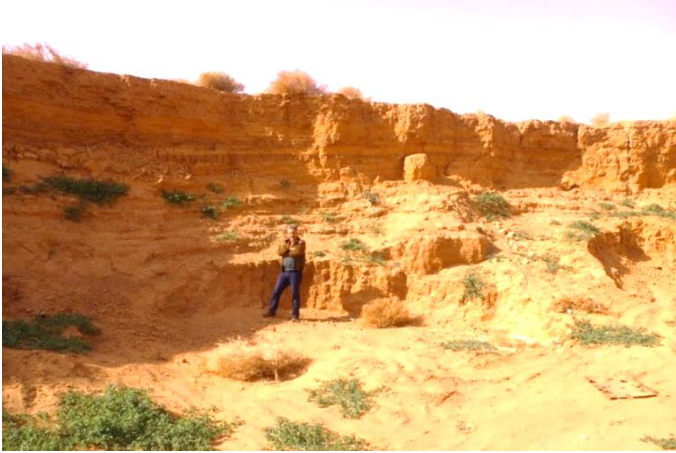
Figure 20: Mud deposit occupying the entire capacity of the Bouchen dam (Photo. Remini, 2018)
