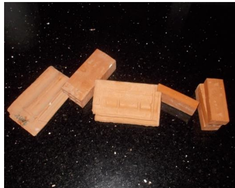
b) Some construction material products produced by the mud of the Foug El Gherza dam (Photo. Remini, 2017)
