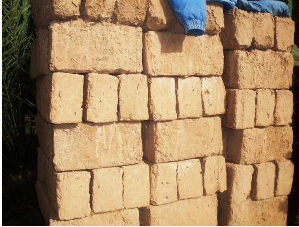
Figure 14: The finished product of Ahbas N'Bouchen's vase ready for construction (Photo. Remini, 2010)
