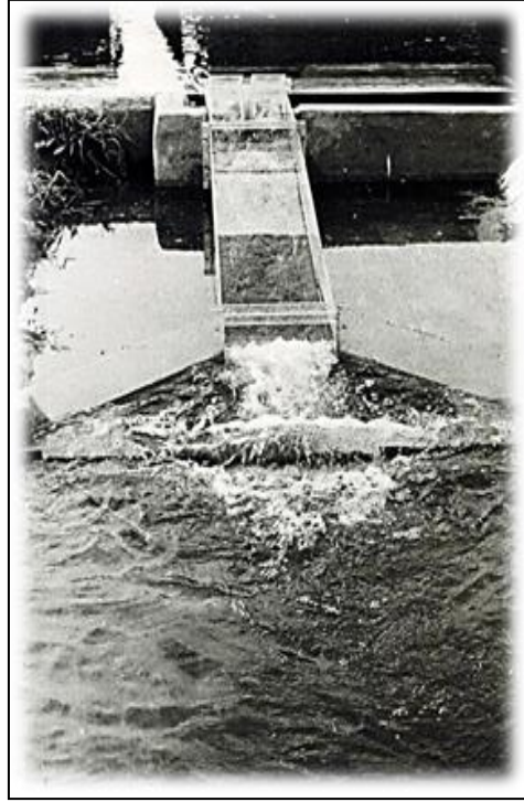
Figure 2: Photo of a model with a swirling flow from the Volga-Don 2 canal.
