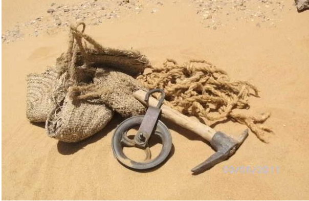
Figure 11: Equipment used for the digging and maintenance of a Foggara (Authors, 2013)
