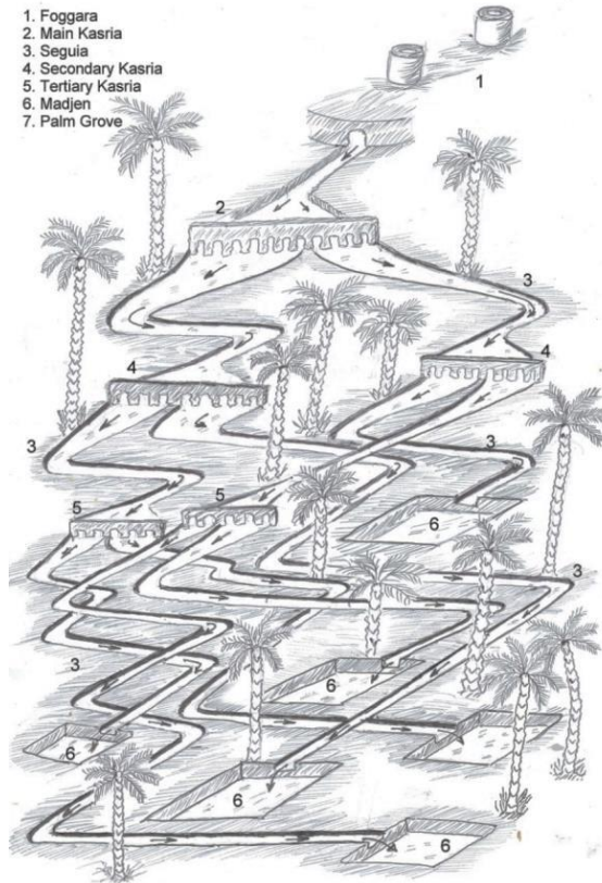
Figure 5: Block diagram of the water distribution network of a Foggara in Touat, Gourara and Tidikelt (Diagram, Remini, 2021)
