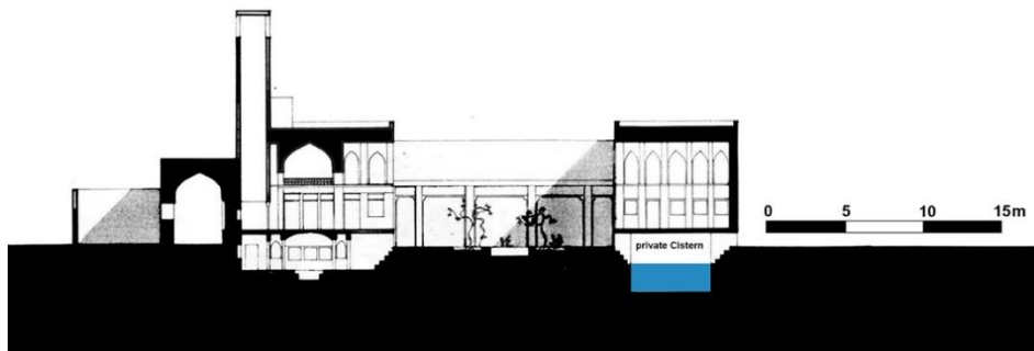
Figure 10: Section of a mansion in Nâsâr neighborhood and its private cistern which was used to supply water for garden and courtyard of the house during the summers. Source: Author based on Tarh-o-Pajouhesh CO., 1974.
