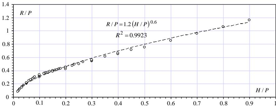
**Figure 5: Graphical representation of  $R/P$  as a function of  $H/P$  and dimensionless relationship**
