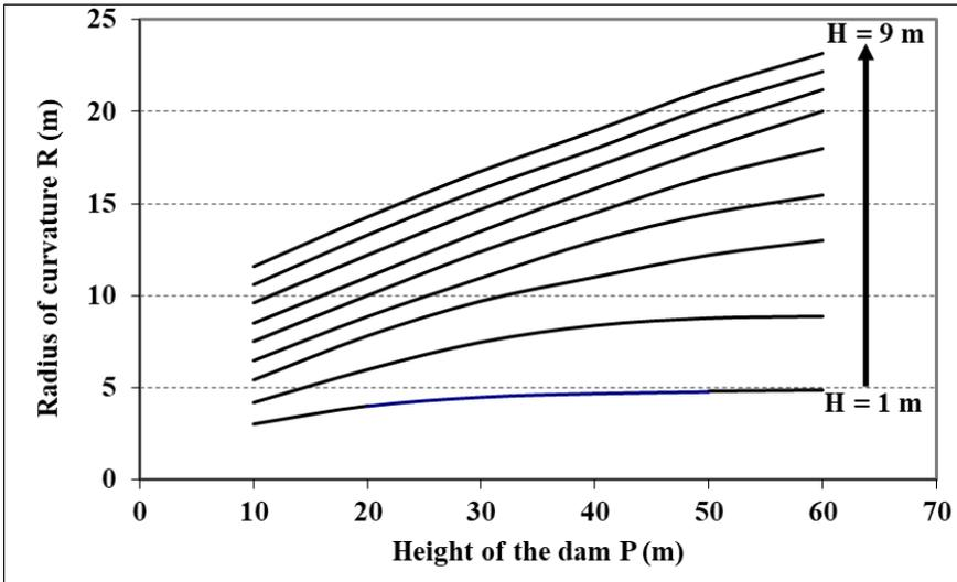
**Figure 4: The graphical representation of the connection radius as a function of the height of the dam corresponding to the head of water over the crest**
