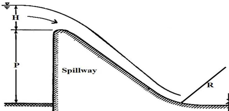
**Figure 1: Sketch of the radius of curvature of the downstream toe of a spillway**
