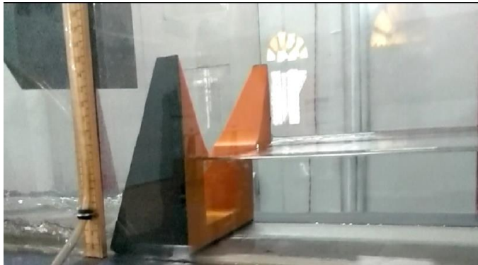
Figure 4: CBC Weir Model Casted with PLA Plastic material fixed inside the tilting flume
