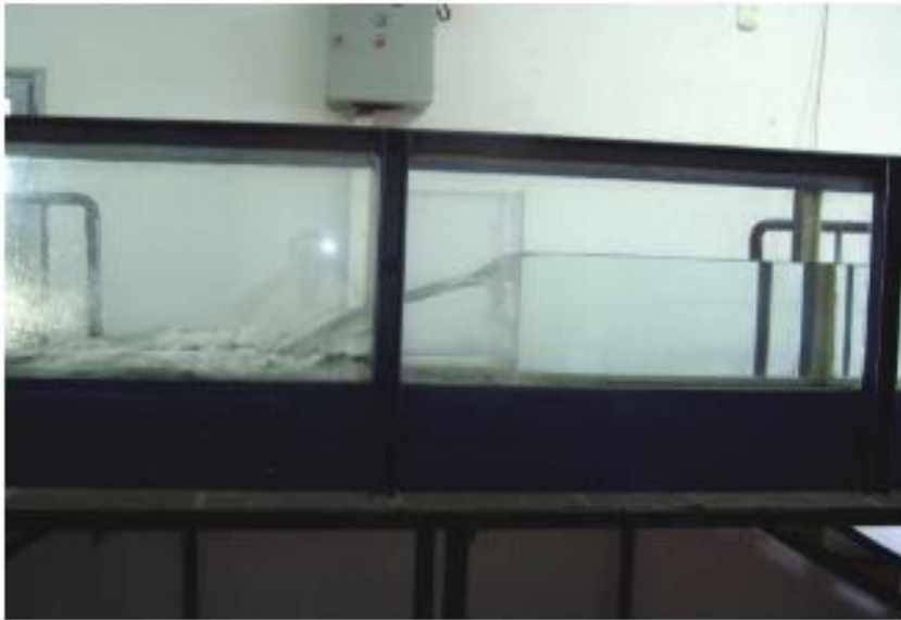
Figure 3: Snapshot of longitudinal profile of the flow upstream and inside the device; flow from right to left.
