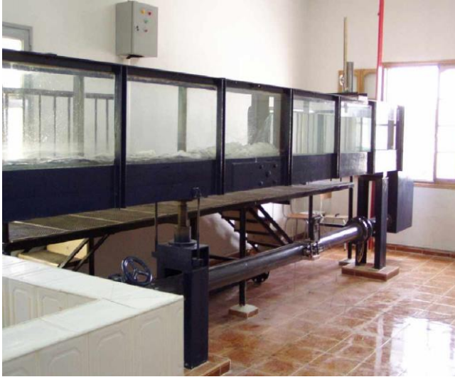
Figure 5: Overview of the rectangular test channel.
