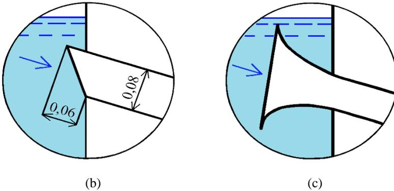
**Figure 3: Principal scheme of model installation: a – with a portal culvert outlet; b - outlet of the "hood" type; c - smooth outlet with vertical rectilinear side walls; 1 to 6 - measuring sections**
