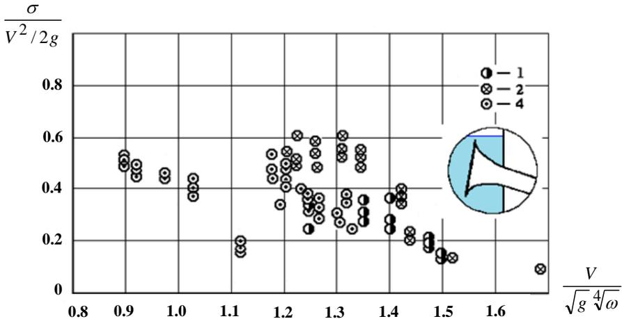
**Figure 7. Pressure fluctuation intensity  $\sigma/(V^2/2g) = f\left(\frac{V}{\sqrt{g} \sqrt[4]{\omega}}\right)$  for the model with a smooth inlet tip: 1, 2, 4 – experimental points in characteristic measuring sections along the syphon culvert axis**
