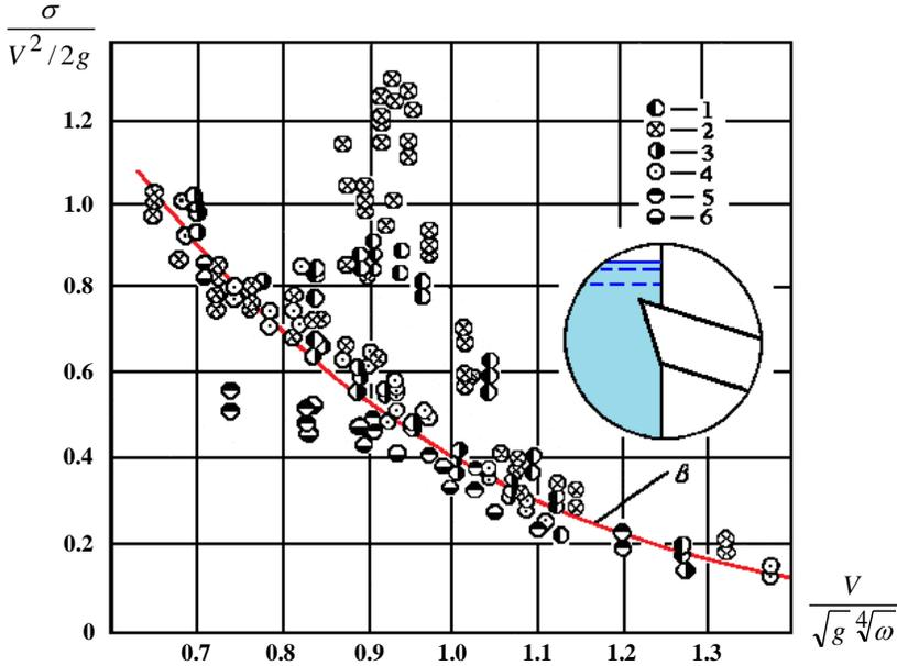
**Figure 5: Intensity of pressure pulsation  $\sigma/(V^2/2g) = f\left(\frac{V}{\sqrt{g} \sqrt[4]{\omega}}\right)$  for a model with an inlet culvert of the “hood” type in the corresponding measuring sections (1 to 6):  $B$  – averaging line for determining  $\sigma$**
