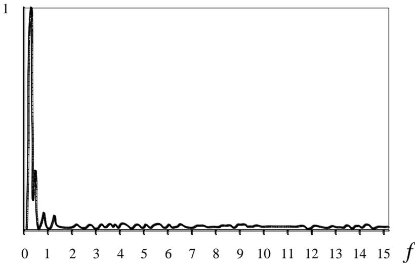
**Figure 8: The normalized function of the spectral density of pressure fluctuations in the second section at  $\frac{V}{\sqrt{g} \sqrt[4]{\omega}} = 1.19$**
