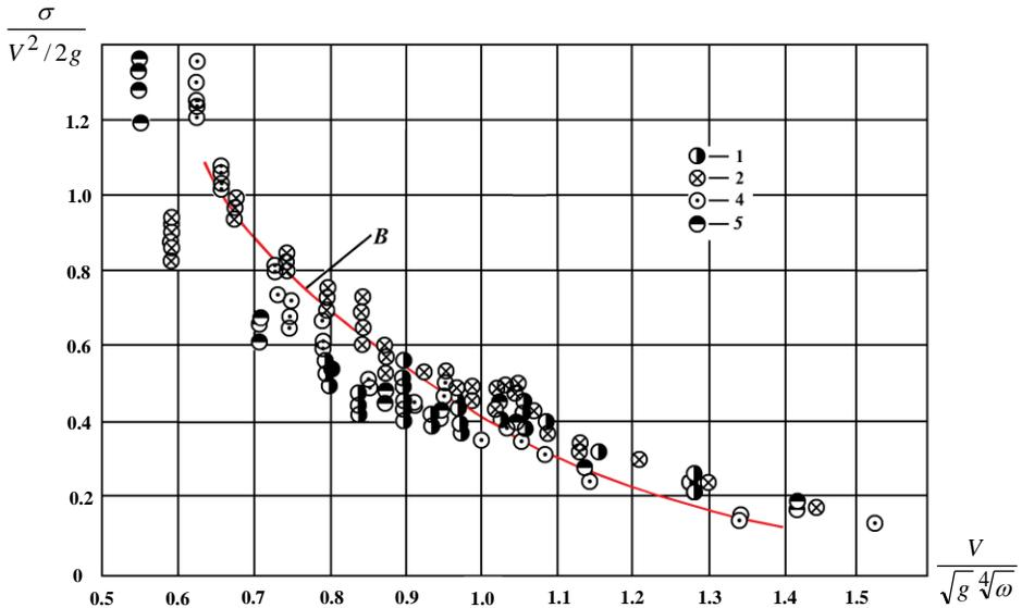
**Figure 6: Intensity of pressure pulsation  $\sigma/(V^2/2g) = f\left(\frac{V}{\sqrt{g}\sqrt[4]{\omega}}\right)$  for the model with a portal inlet culvert: 1 to 5 – experimental points in the corresponding measuring sections along the axis of the inverted syphon pipe; B - averaging line from Fig. 5**
