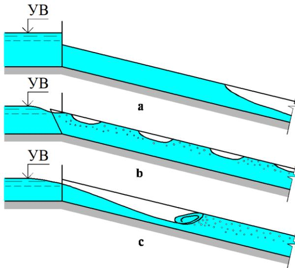
**Figure 4: Transitional modes of flow in the initial section of the syphon culvert: a - the first transitional mode: b - the second transitional mode with a self-loading portal of the "hood" type: c - the second transitional mode with a non-self-charging portal culvert inlet**
