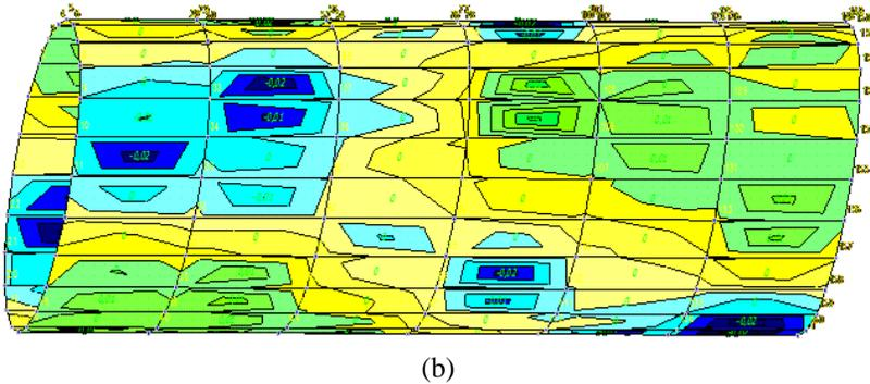
**Figure 2: An example of the formation of a defect in the syphon pipes [4]: a - outside the long-term operated Tashlinsky syphon on the Pravo-Egorlyk Canal; b - diagram of excess equivalent stresses according to von Mises in the places of defect formation**
