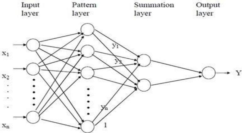
**Figure 8: Schematic of the GRNN**
