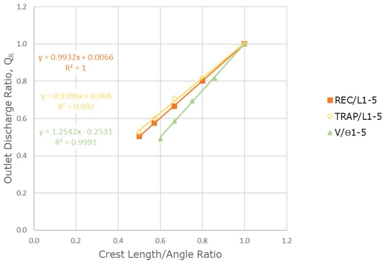
**Figure 5: Outlet discharge ratio versus crest length or angle ratio for different weir shapes**
