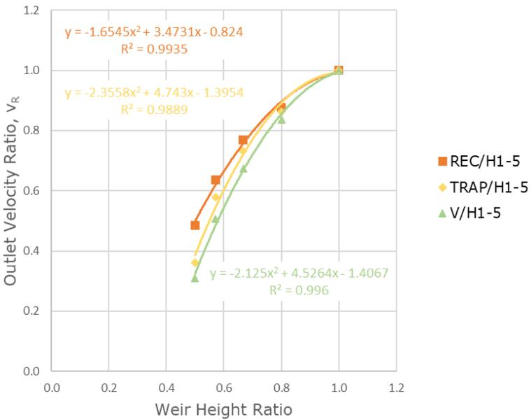
**Figure 6: Outlet velocity ratio versus weir height ratio for different weir shapes**
