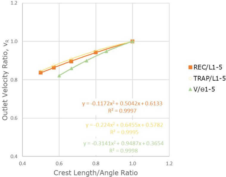
**Figure 7: Outlet velocity ratio versus crest length or angle ratio for different weir shapes**
