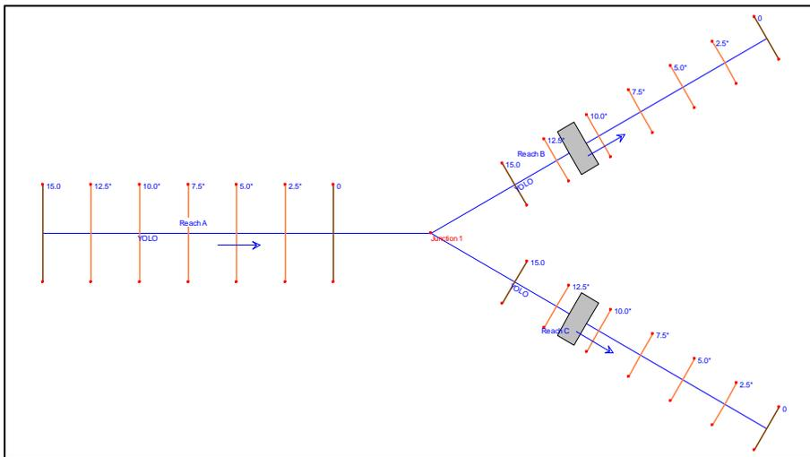
**Figure 3: Overall layout with weirs of the reaches in HEC-RAS setup**
