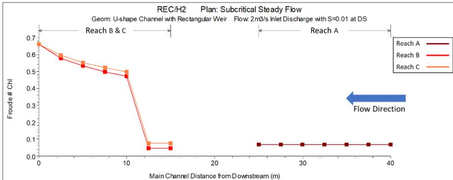
Figure 10: Froude number versus main channel distance for REC/H2
