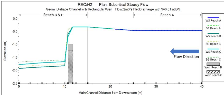
**Figure 9: Water elevation versus main channel distance for REC/H2**
