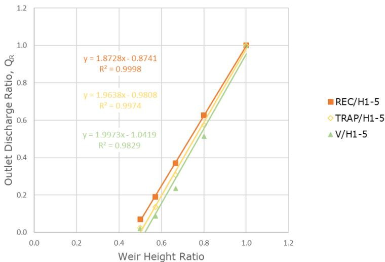
**Figure 4: Outlet discharge ratio versus weir height ratio for different weir shapes**
