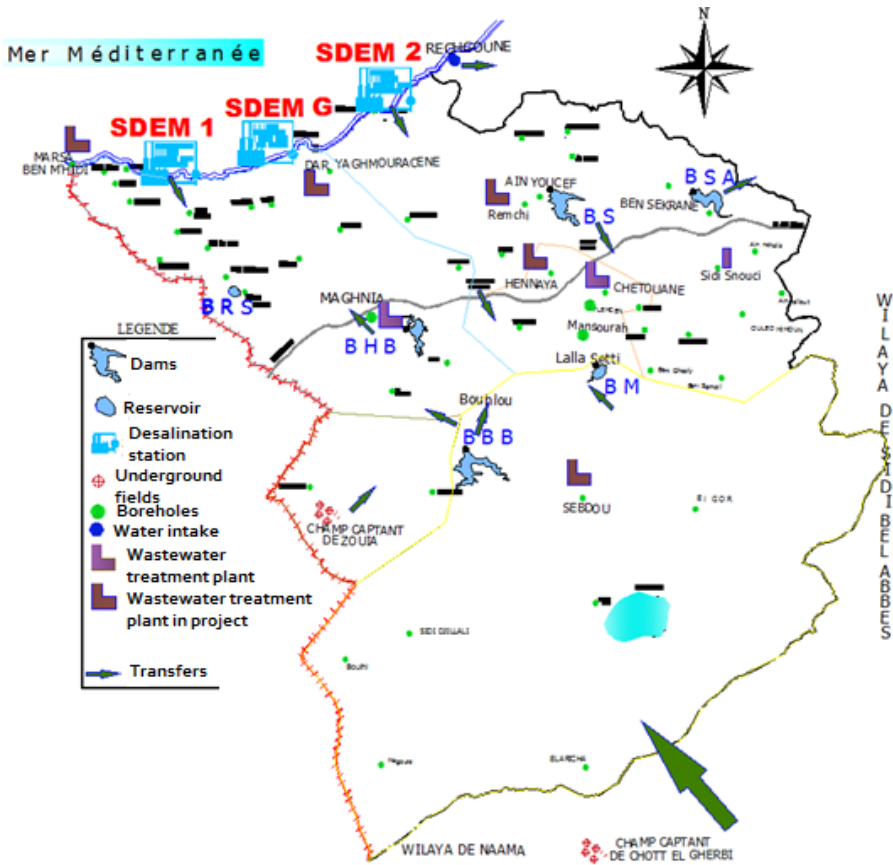
Figure 4: Components of the Tafna water resources system
