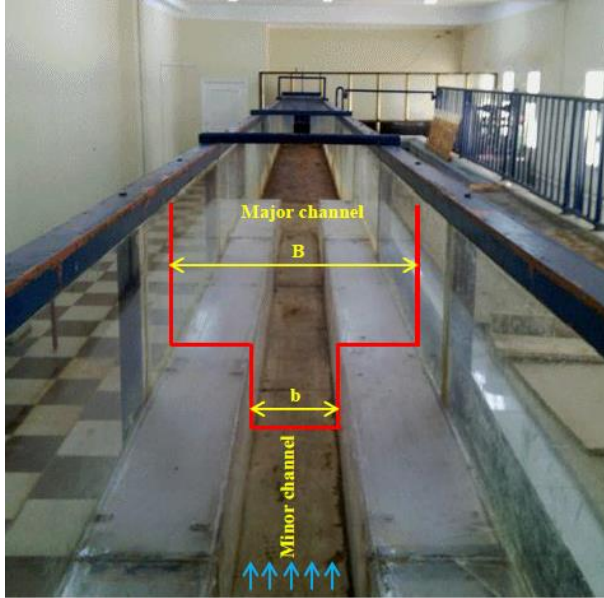
Figure 1: Compound rectangular section measurement channel
