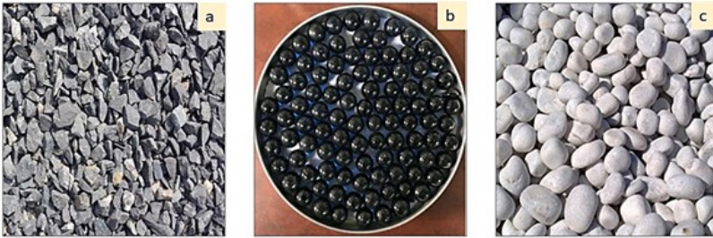
Figure 5: Different energy storage materials: (a) black granite, (b) black glass balls and (c) marble stones (Mevada et al., 2022)
