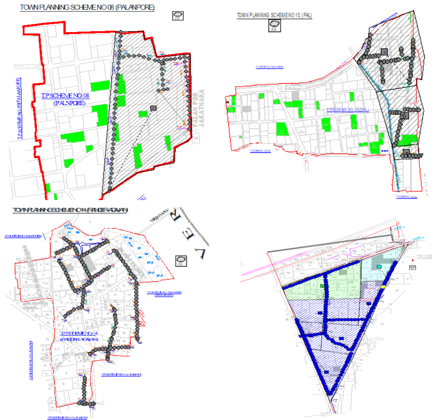
Figure 4: TP Scheme 8, 10, 14 & 46 (Palanpore, Pal, Rander-Adajan & Jahangirpura) drainage plan in the SWMM model
