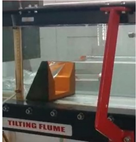
Figure 3: CBC Weir Model Casted with Poly Lactic Acid Plastic material
