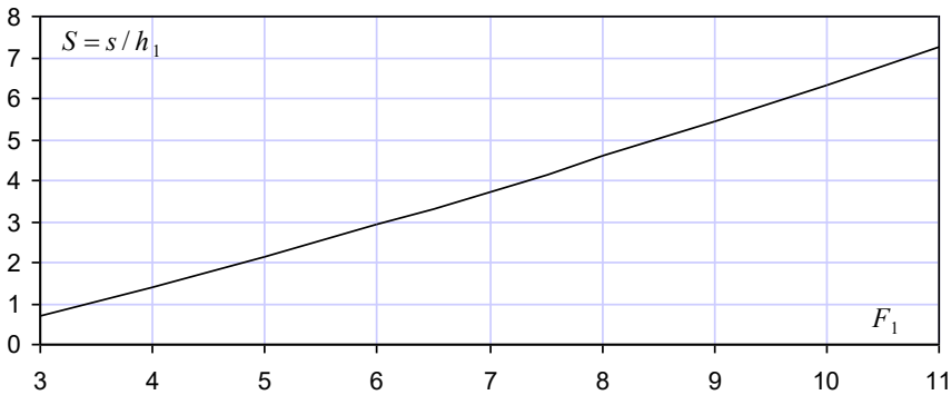
Figure 2: Variation in the relative sill height S as a function of F_1 according to Table.1
