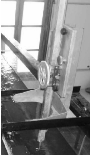
Figure 11: View of the double-precision Vernier point-gauge used for the depth measurement
