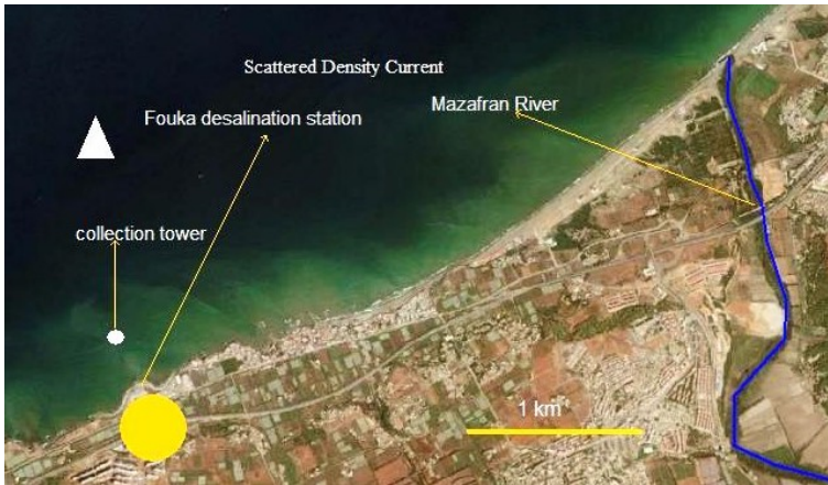
Figure 19: Density current propagates toward the site of the capture tower of the Fouka seawater desalination station (Google Earth)
