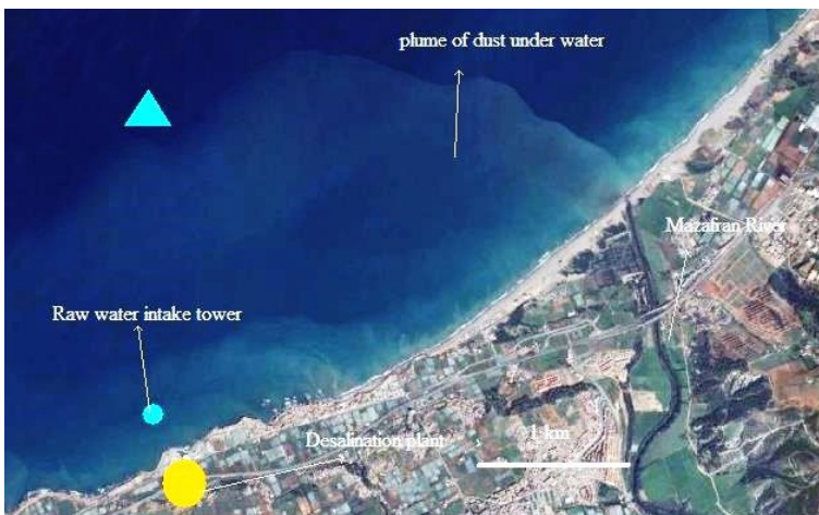
Figure 20: Current of less dense density propagates toward the site of the capture tower of the Fouka seawater desalination station (Google Earth)
