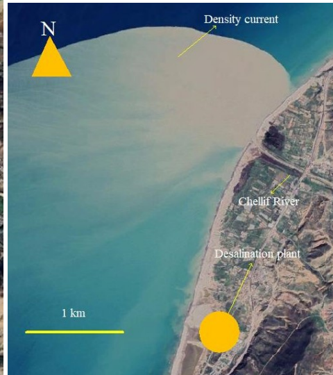
Figure 18: Vanishing of a density current just after its formation due to sea currents that move in the opposite direction of propagation of the density current (Google Earth)
